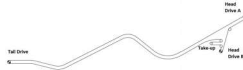
Figure 7 - Conveyor CV-003 drive and take-up arrangement.
