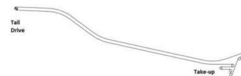
Figure 3 - Conveyor CV-002A drive and take-up arrangement.
