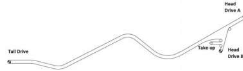
Figure 7 - Conveyor CV-003 drive and take-up arrangement.
