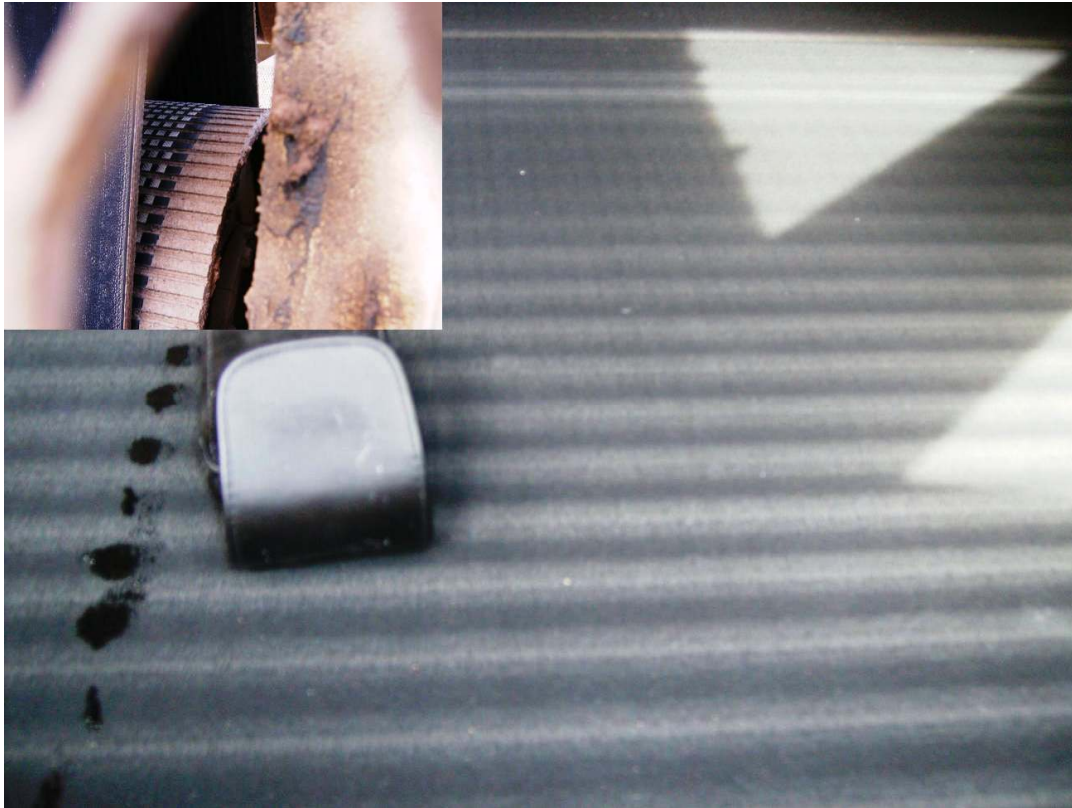
Figure 9. Belt Cover Wear From Sharp Ceramic Lagging Tile. The lagged pulley surface is shown in the upper left corner.
