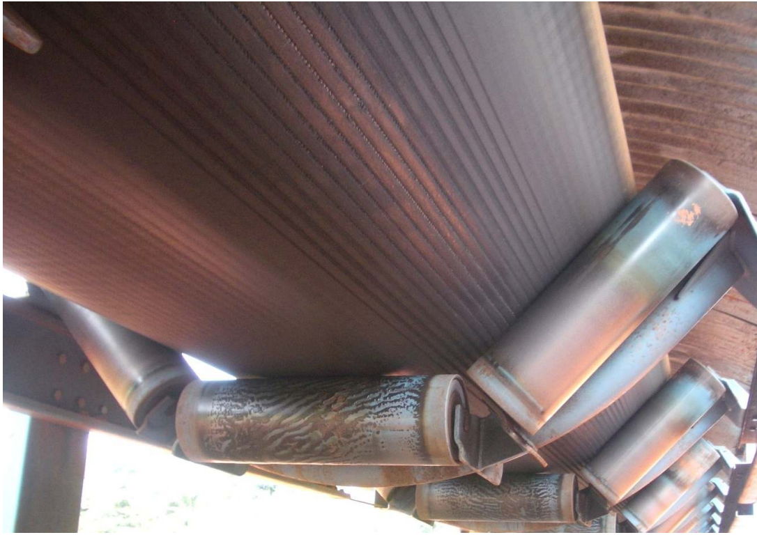
Figure 8. Belt Cover Wear Due to Idler Forward Tilt
