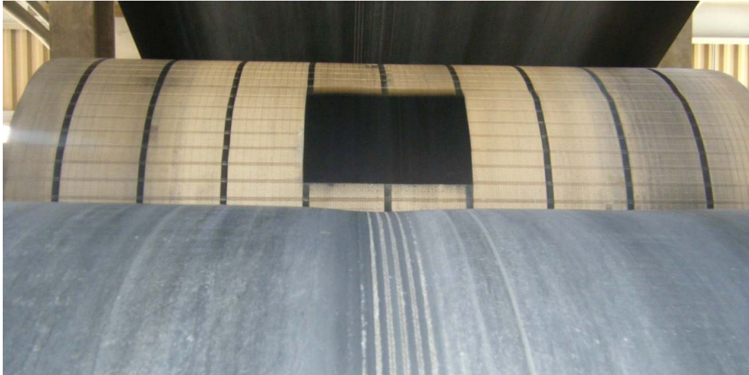
Figure 11. Bottom Cover Wear From Ceramic Lagging
