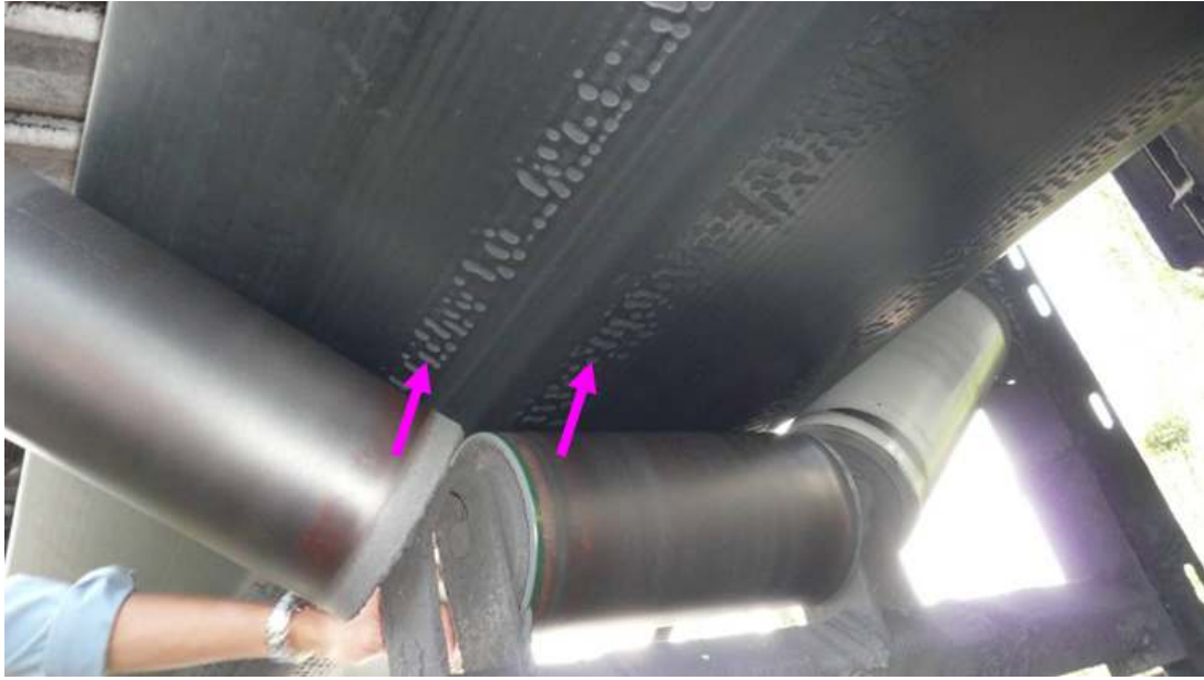
Figure 7. Bottom Cover Damage at High Contact Pressure Area
