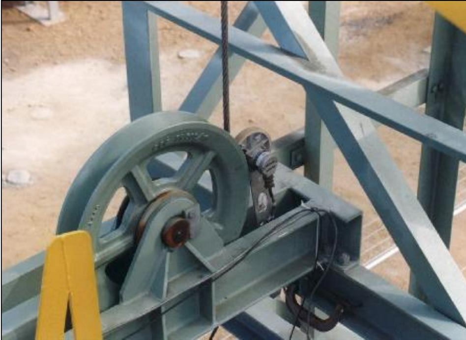
**Figure 11:** *Take-up displacement – Optical encoder mounted on take-up sheave*
