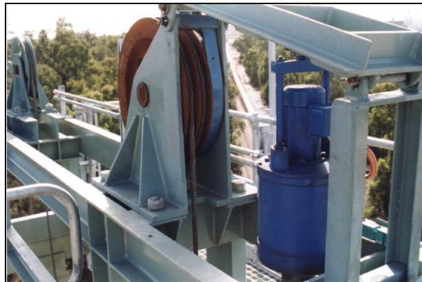
FIGURE 3 – A capstan installed using a disk brake FIGURE 4 – A capstan installed using a band brake
