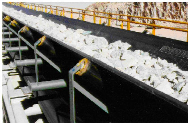
Figure 1 - Large Particles (Ore) on Conveyor Belt
