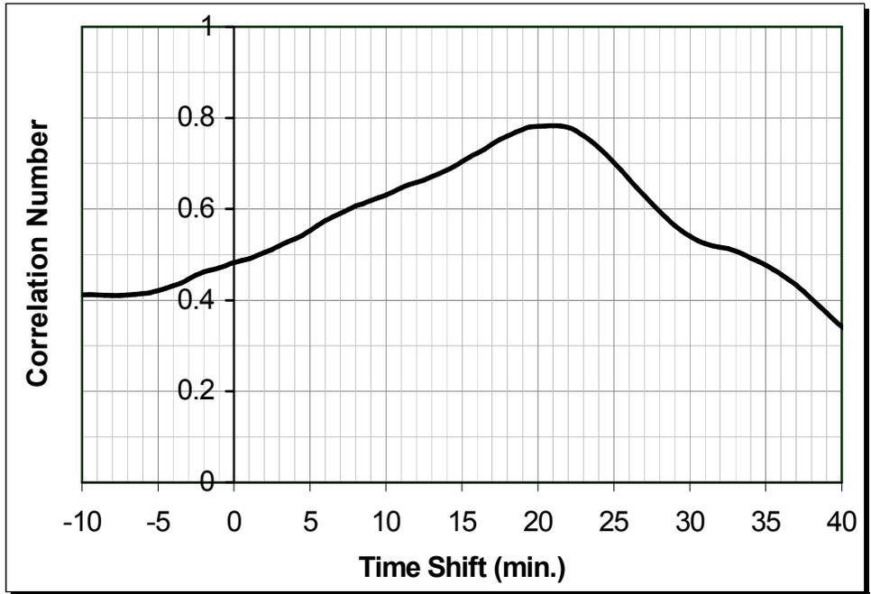
Fig. 15: Phase Shift between Circuit Feed Rate and Product Size
