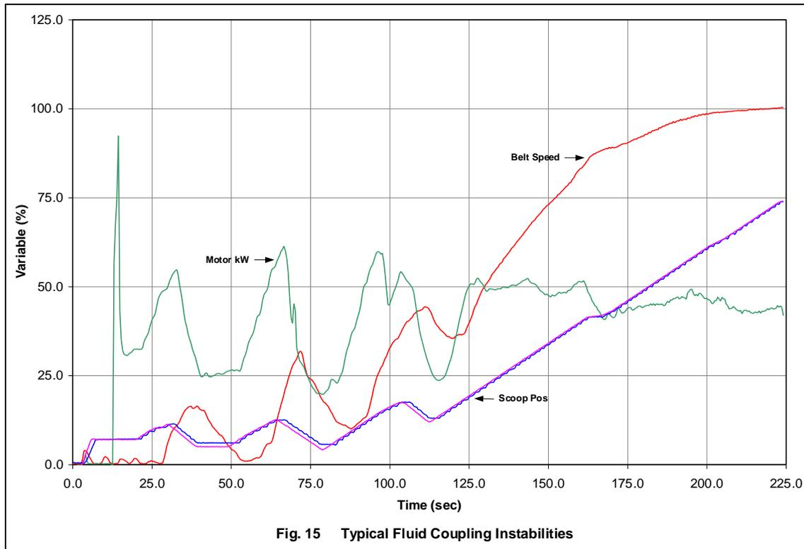
Fig. 15 Typical Fluid Coupling Instabilities
