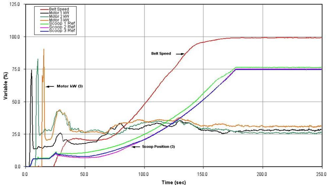
Fig. 10 Preemptive Fluid Coupling Controls - Empty Conveyor Start - MRN Project
