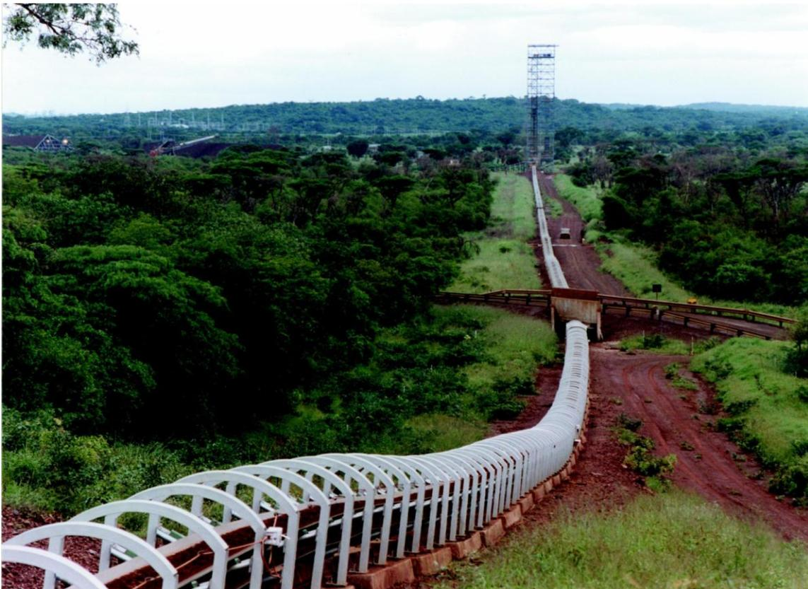
The 8.9 km curved K2 conveyor at the Ingwe mine in Middleburg, South Africa also uses head and tail inverter drives. The overland system includes three conveyors in a 13.4 km route. Conveyor K2 has regenerative sections and is driven by two head drives (630 kW and 315 kW) and a single tail drive (315 kW). Siemens manufactured all the inverters.
