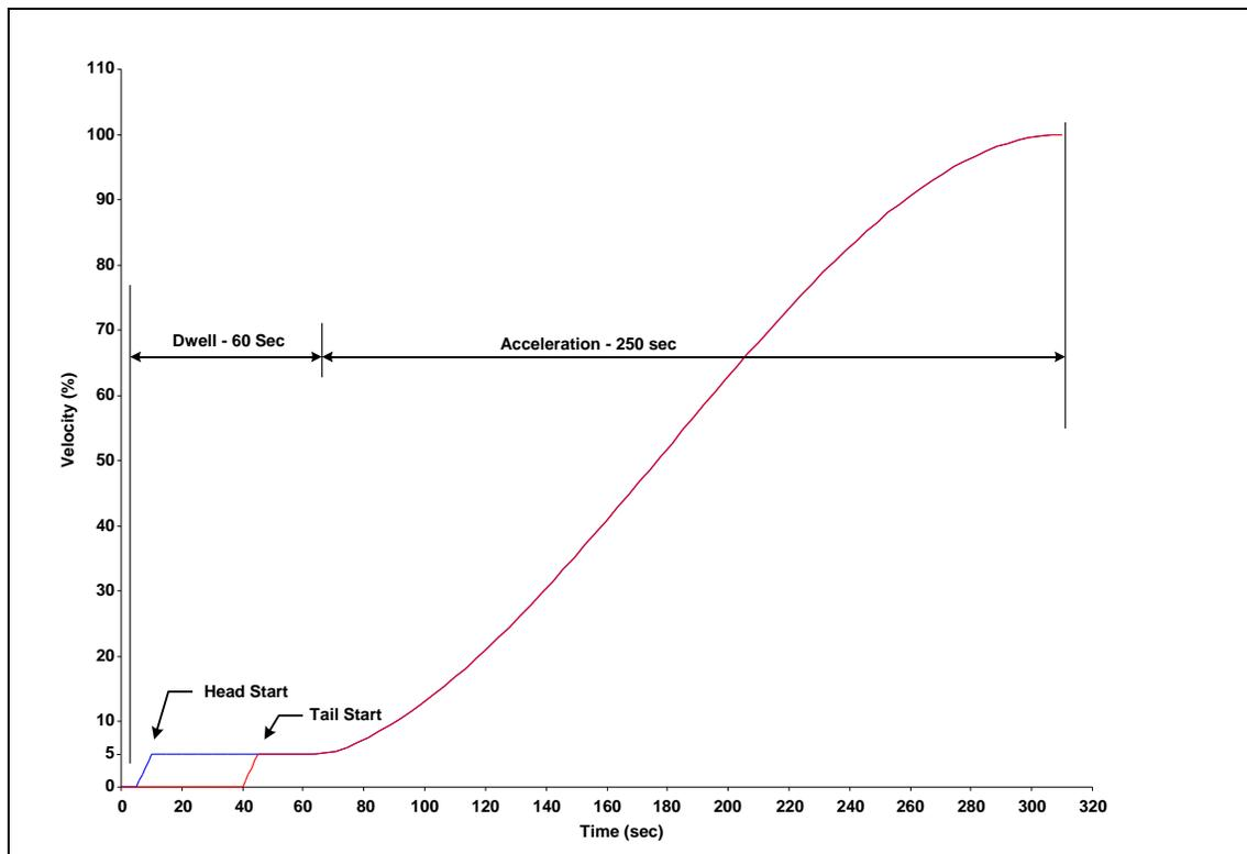
Fig. 8 Adaptive Fluid Controls - Conveyor Start Sequence - Indo Kodeco Project
