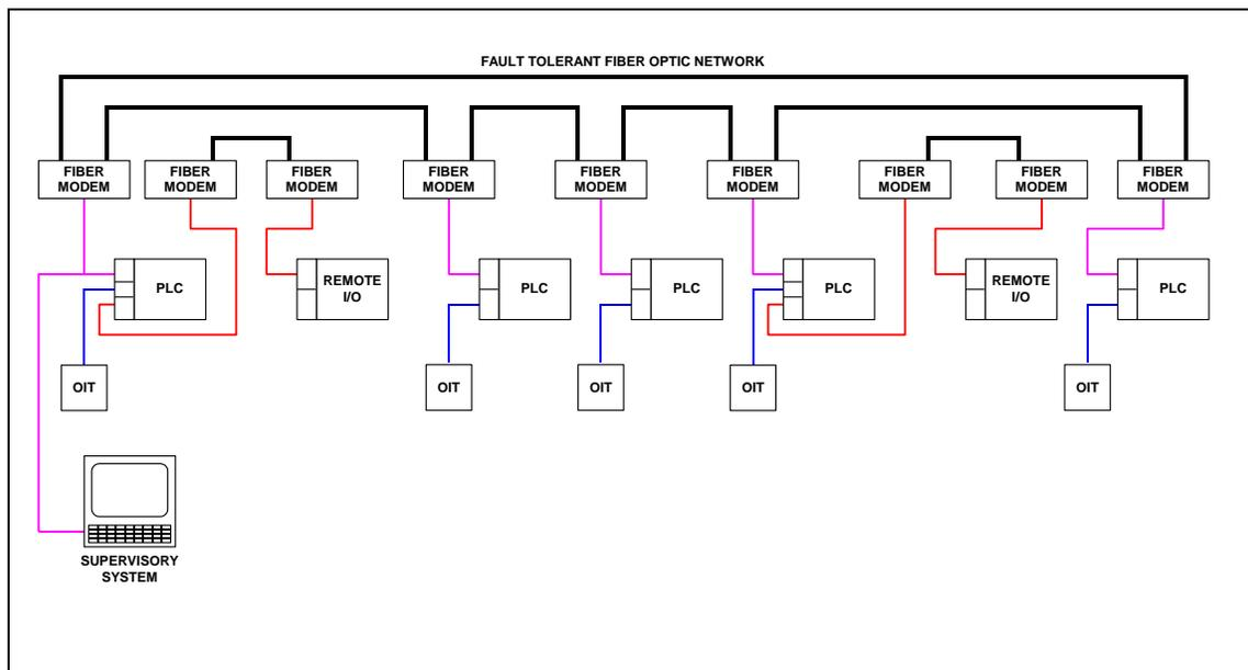
Fig. 6 Typical Mixed Network Architecture - Pico Project
