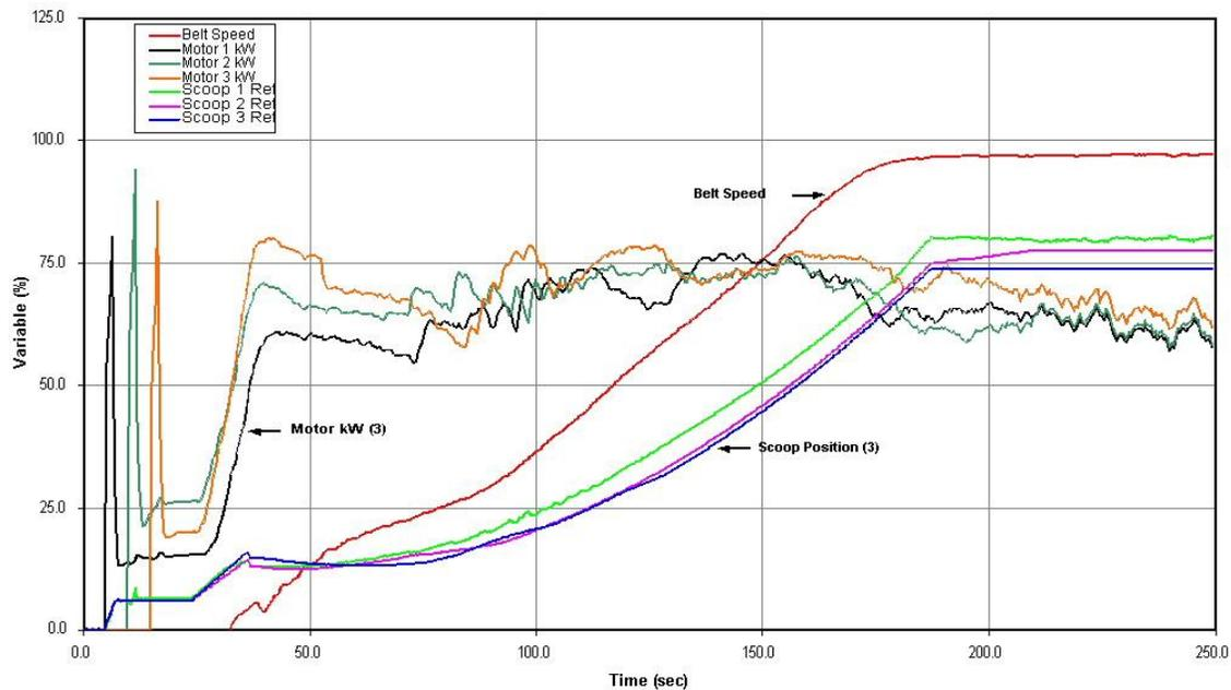
Fig. 9 Preemptive Fluid Coupling Controls - Loaded Conveyor Start - MRN Project
