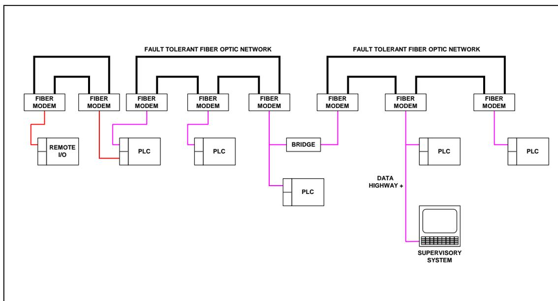
Fig. 5 Typical Peer-to-Peer Network Architecture - Indo Kodeco Project
