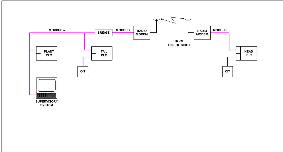
Fig. 4 Typical Serial Link Network Architecture - Zisco Project
