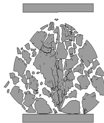
Figure 2. Impact fracture of single particle – magnitude 4X.
