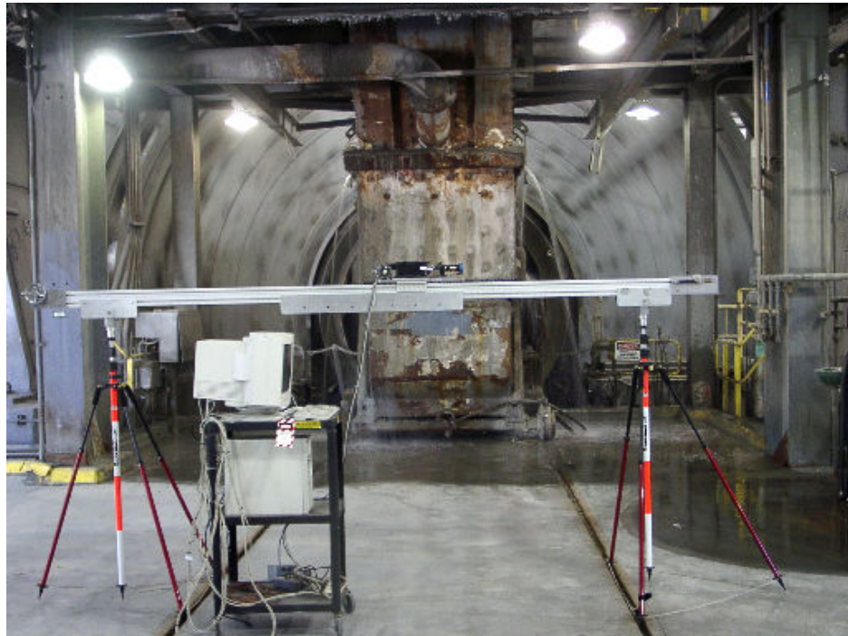
Figure 11. – Mill Laser Scanner fully assembled – 4 meter bar length
