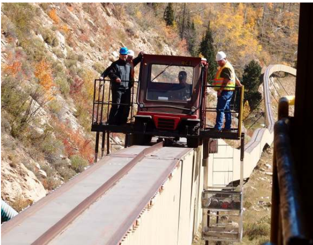
Figure 5. Using Modified All-Terrain Vehicle as Trolley
