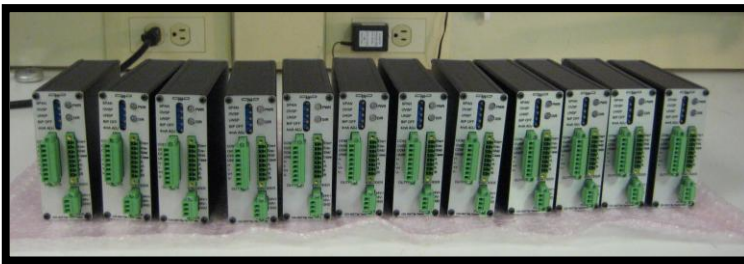
(Top) DEFT3A Tachometers ready for calibration and shipping (Right) DEFT3a Tachometers installed for redundancy and conveyor slip detection
